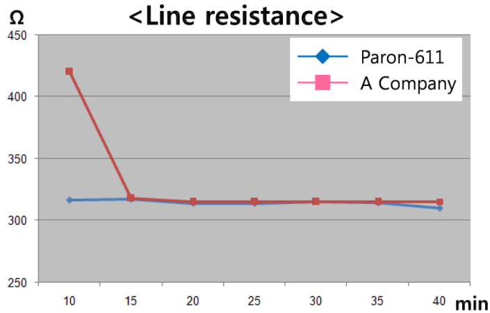
Resistance of various curing times at a fixed temperature, 150°C
