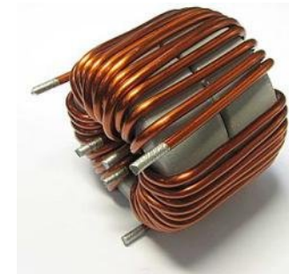
Boost Inductor : CSC HighFlux Material : Toroidal Core
