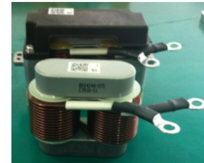
PFC Inductor, Noise Filter : CSC MegaFlux, SENDUST, HighFlux Material : Toroidal Core or Other Special Shape Core
